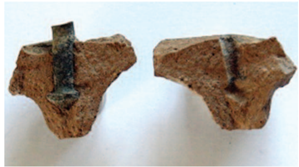
Fig.4. Reused rivets in cement from Ash-next-Sandwich. (photo: © author)
